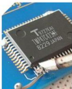
Repair drag welding
