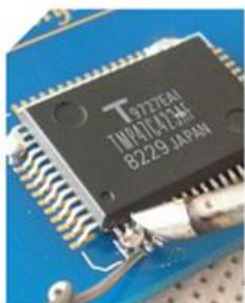
Repair drag welding
