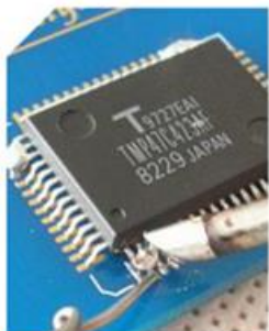
Repair drag welding
