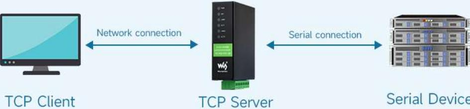
TCP Server will be listening configured ports and waiting for TCP Client connections, data from the serial device will be transferred via TCP Server to every connected clients
