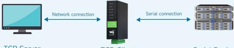
TCP Client will try establishing TCP connection with configured IP to achieve bi-directional transparent transfer between the server and serial device, and keeps retrying if failed
