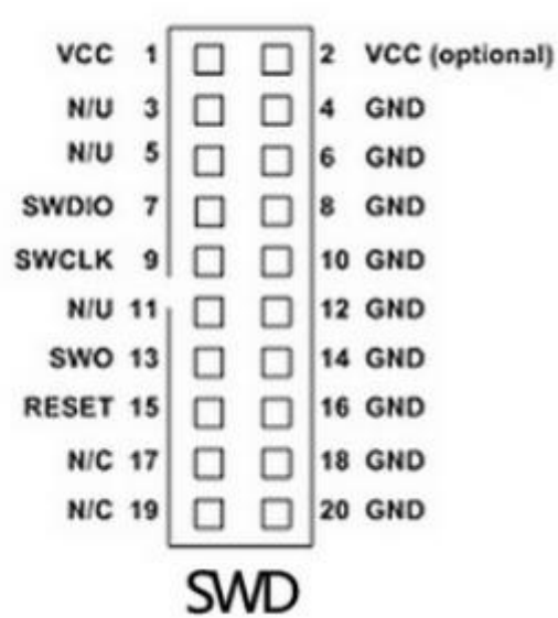
Figure 2. SWD Header Pinout
