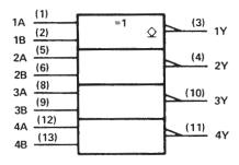
positive logic:  $Y = \overline{A \oplus B} = AB + \overline{AB}$
