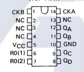
SN5493A, SN54LS93 . . . J OR W PACKAGE SN7493 . . . N PACKAGE SN74LS93 . . . D OR N PACKAGE (TOP VIEW)
