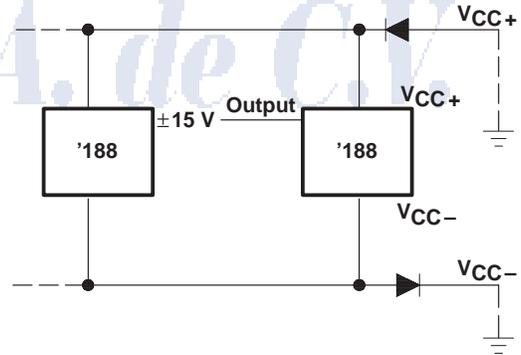
Diodes placed in series with the  $V_{CC+}$  and  $V_{CC-}$  leads will protect the SN55188/SN75188 in the fault condition in which the device outputs are shorted to  $\pm 15\text{ V}$  and the power supplies are at low voltage and provide low-impedance paths to ground.
