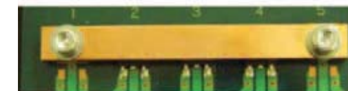
Heat sink is mounted 66mm x 7.3mm x 3.0mm
