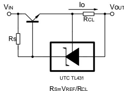
$$R_s = V_{REF} / R_{CL}$$
