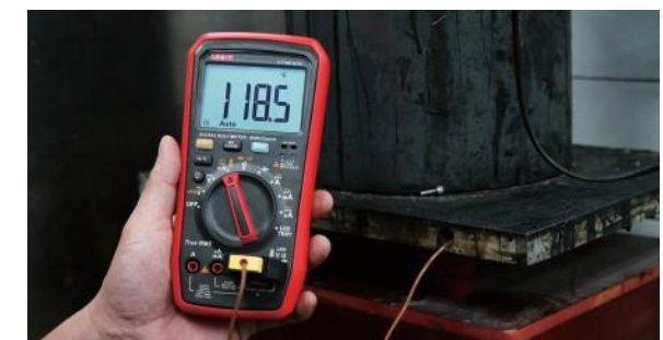
Temperature measurement (UT17B/18B MAX)
