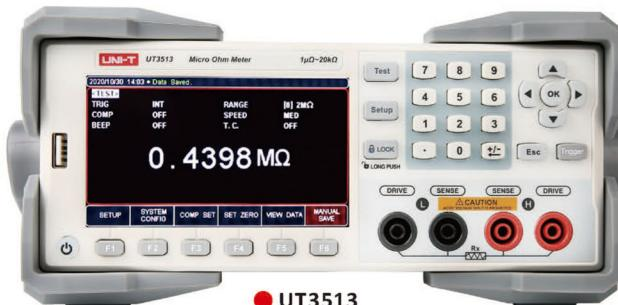
The UT3510 Series Micro Ohm Meters contain 2 models: UT3513 and UT3516, which can be used in professional sorting function, and can judge HI/IN/LO for resistance. The result can be displayed on screen, indicated by buzzer and external I/O output. With enhanced PC remote-control instruction set and compatible with SCPI, the instrument can efficiently process remote-control and data collection function.
