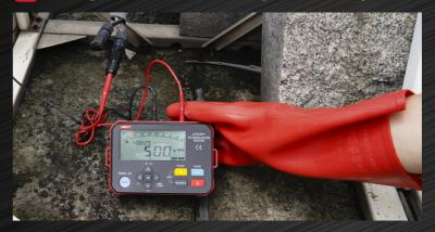
The maximum rate voltage between terminals is DC 1000V. Do not measure any energized equipment with a voltage of over DC 1000V, otherwise, it can cause electric shock or fault.
