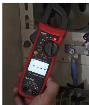
NCV multi-segment display and audio/visual alarm
