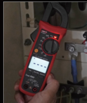
NCV multi-segment display and audio/visual alarm
