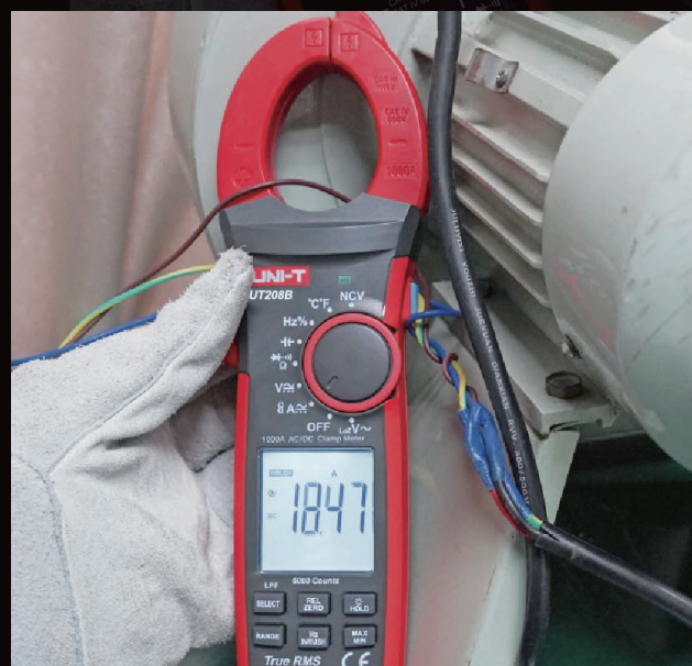
Inrush current capture (UT206B/207B/208B)
