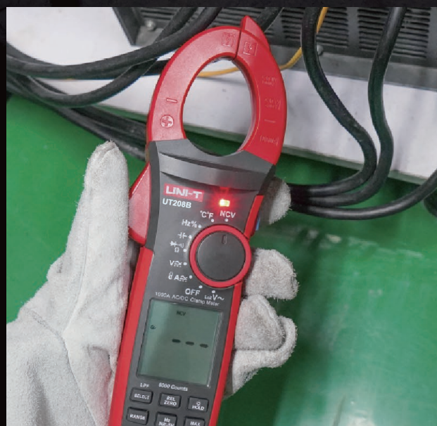
NCV Multi-Segment Display and audio/visual alarm
